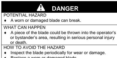
Replace a worn or damaged blade. ٠
